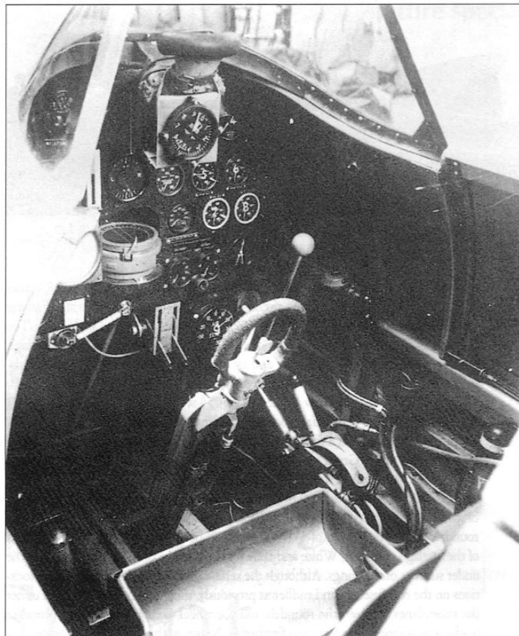
Close-up of the cockpit interior after the armament had been fitted circa early 1937 – note the gun firing lever in the centre of the spade grip control column (R J Mitchell Museum)
