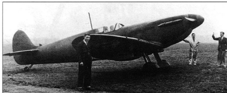
K5054 as she emerged from the Eastleigh workshops after being camouflaged in September 1937. Note the ejector exhaust manifolds now fitted (Vickers)
