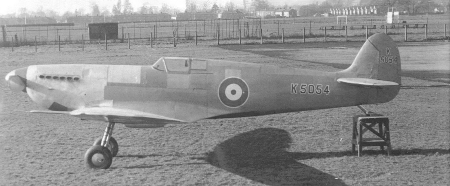
The Spitfire prototype, K5054, then known as the F.37/34, as she looked immediately prior to her first flight on 5 March 1936. Note the unpainted natural metal finish, unfaired main undercarriage legs with solid mainwheel hubs and the initial design, 'angled' horn balance rudder (Vickers via Mike Jerram)
